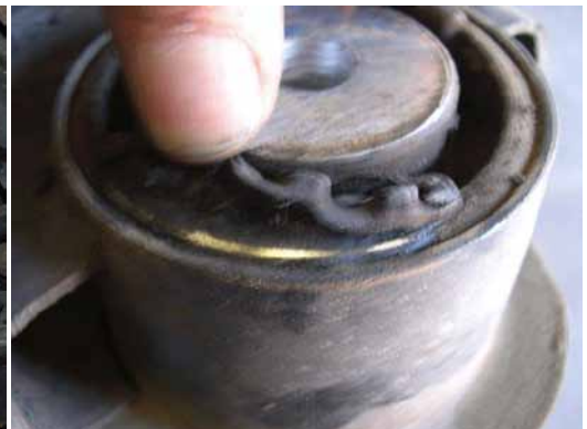
The control surface of the bush is torn from normal wear.
