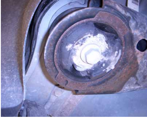
This is a salt caused failure on a Dodge Charger used by an Indiana Sherriff's Department.
