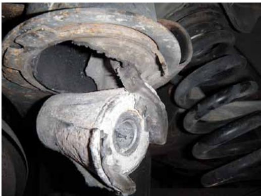
This is caused by road salt corroding the aluminium ferule. This is a complete total falling out of the car failure
