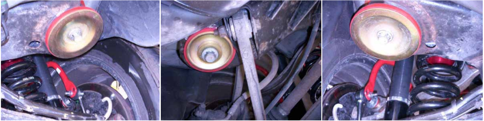
Pedders EP1172 Bushes Installed on the Cass County Car
