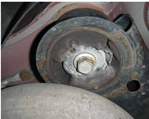
This is caused by road salt corroding the aluminium ferule. This is a complete total falling out of the car failure
