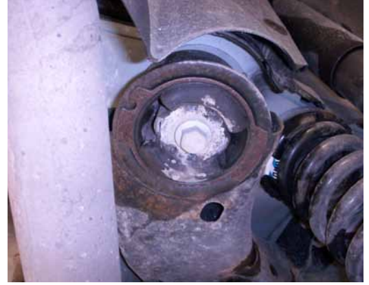
Cass County Sheriff Second Failed Bush by Corrosion
